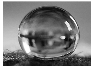
Figure 4. Collared water droplet (diameter \sim 2 mm) over a superhydrophobic cotton textile after its coating with perfluorinated MWNTs.
